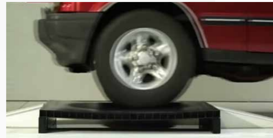
Load case: Jeep with one wheel on a 1 m x 1 m panel.
